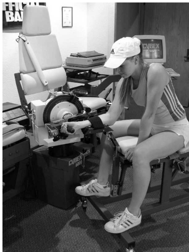
Figure 1 Isokinetic testing set-up for wrist flexion/extension with the Cybex 6000 dynamometer. Informed consent was obtained for publication of this figure.
