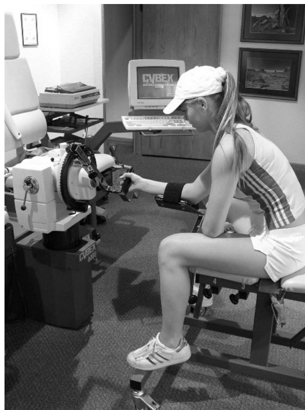
Figure 2 Isokinetic testing set-up for forearm pronation/supination with the Cybex 6000 dynamometer. Informed consent was obtained for publication of this figure.
